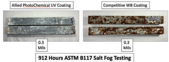
Picture 6: ASTM B117 Salt Fog – 912 hours UV vs water-based at 0.3 mils dry film thickness
