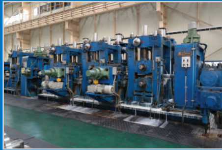
4" ~ 8" O.D, Up to 18mm wall thickness TUBE MILL LINE
