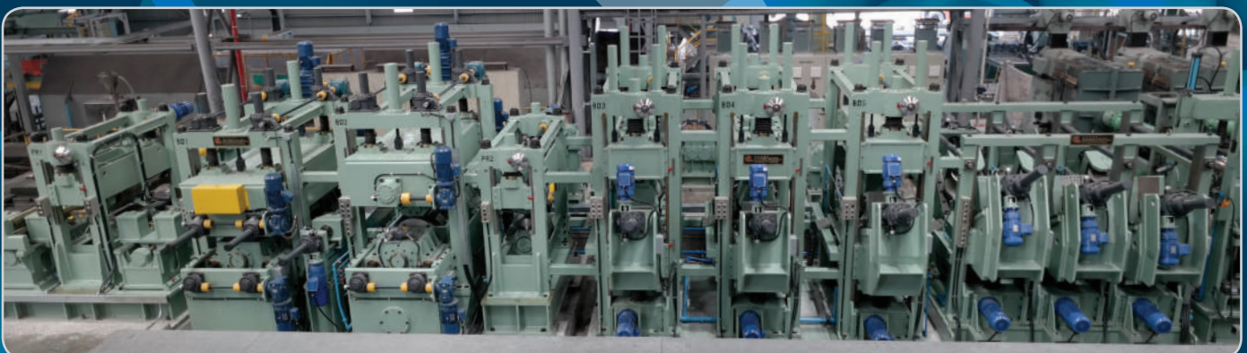
12" ~ 24" O.D, Up to 20mm wall thickness TUBE MILL LINE
