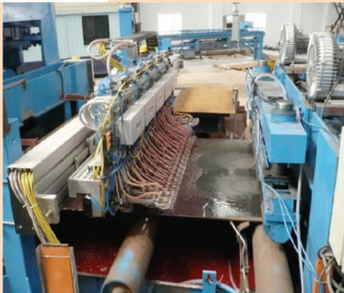
Spiral mill 2 m coil - Thickness 5 – 25 mm
