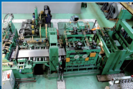
5" ~ 12" O.D, Up to 16mm wall thickness TUBE MILL LINE
