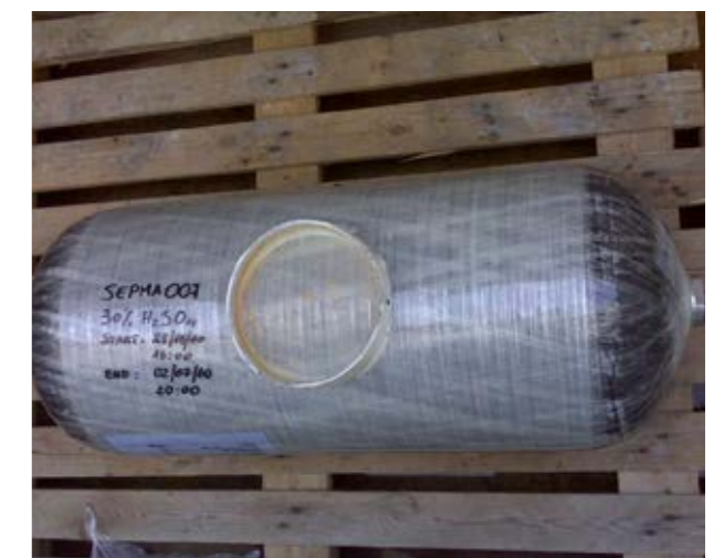
Acid attack test
