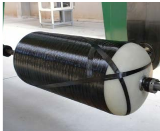
Production a type IV Cylinder
