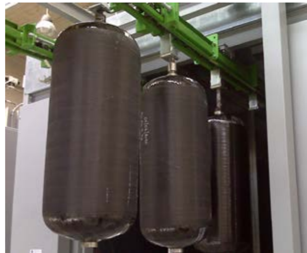
Curing a type IV Cylinder
